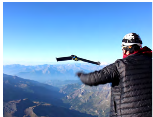
Figure 6-42: UAV systems for GIS typically include flight-planning utilities to specify adequate image overlap and approximate positioning (courtesy senseFly Ltd.).
