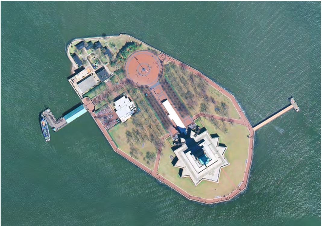
Figure 7-14 An example of a High Resolution Orthophotograph (HRO), distributed by the U.S. Geological Survey. Individual persons can be identified near the flagpole in the upper left part of the island, as well as the statue and shadow to the lower right.
