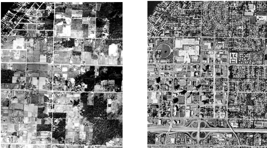
Figure 14-2: Spatial data may be in error because of the passage of time. Road maps based on 1936 photographs (left) from the city of Bellevue, Washington, are likely to be in error in 1997 (right). (courtesy Washington Department of Natural Resources).
