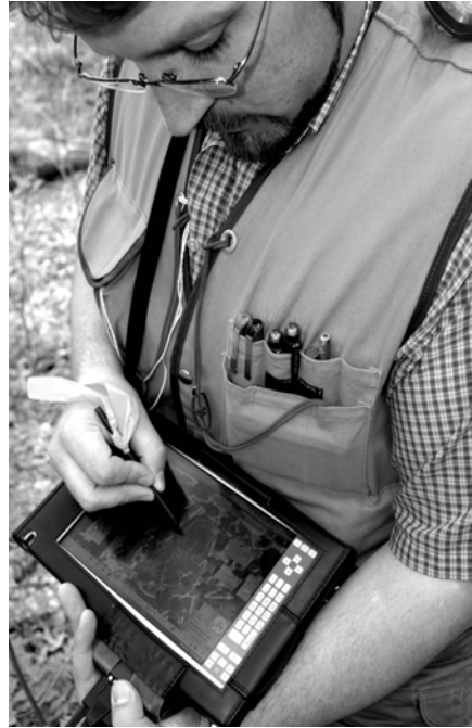
Figure 5-29: Ruggedized tablet computers may be carried in the field and used for data entry. Large screens allow efficient display and field editing of spatial data.
