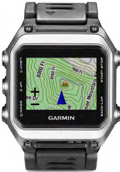
Figure 15-2: Miniature GNSS receivers are available to record speed, distance, and log tracks, that may later be downloaded and analyzed (courtesy Garmin Inc.).
