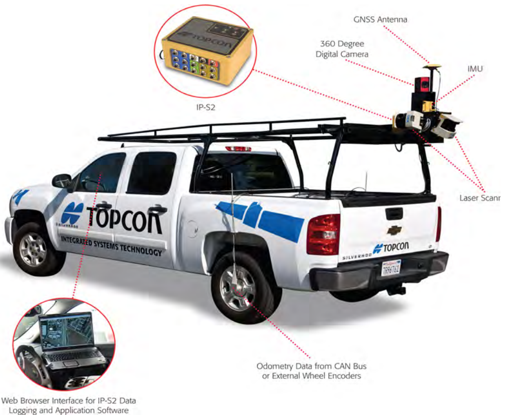
Figure 15-5: Mapping systems combined with GNSS, three-dimensional imaging lasers, optical imaging systems, and other measurement systems to provide integrated three-dimensional measurements in real time (courtesy Topcon).
