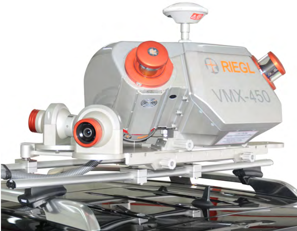
Figure 15-4: Portable, 3-dimensional scanners are in large-scale production, and allow rapid, accurate collection of x, y, and z positions along with image and other data (courtesy Riegl Systems).
