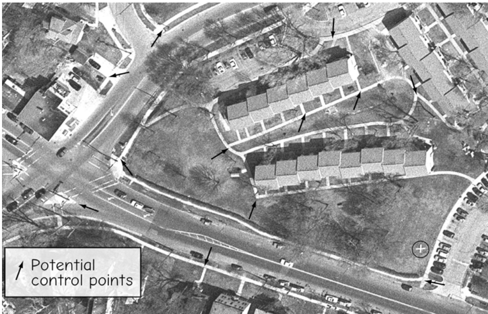
Figure 4-29: Potential control points, indicated here by arrows, may be extracted from digital images that have been geometrically corrected to provide an accurate, coordinate-projected rendering.
