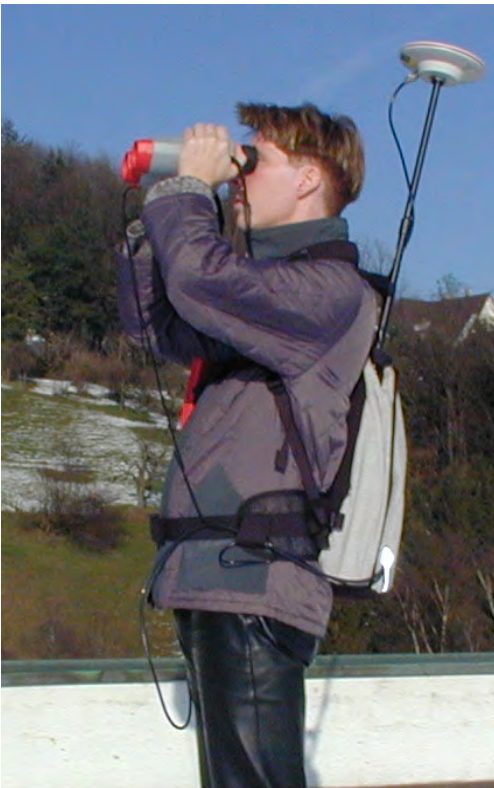
Figure 5-34: A laser rangefinder may substantially improve the efficiency of field data collection with GPS. Here, a system integrates a binocular unit to automatically calculate positions from GPS measurements and distance and angle observations. Also note the range pole to raise the GNSS antenna above the collector's head (courtesy Leica Geosystems).
