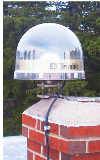
Figure 3-19: A Continuously Operating Reference Station (CORS), used to collect high-accuracy positional measurements from satellites for modern datum development. (courtesy NOAA).
