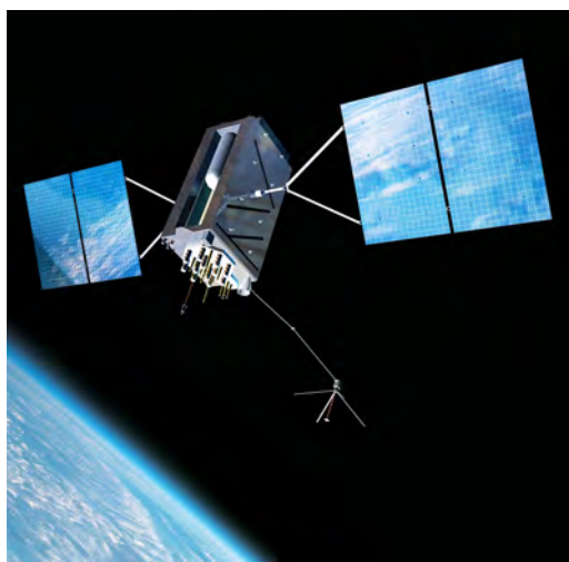
Figure 5-1: An artist's rendering of a Galileo satellite, part of a planned 30-satellite constellation at the heart of a European Union–led satellite navigation system (courtesy Lockheed Martin).
