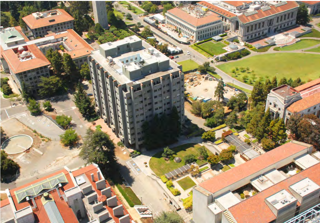
Figure 15-11: An example of extremely high-resolution LiDAR and image coordinate data. This is a combination of multiple image views to create a three-dimensional data set of an area on the U.C. Berkeley campus. These are real data, and not generated animations, created from subcentimeter-resolution x, y, z data. Image data provide color information and LiDAR data location and texture for every point, allowing lifelike renditions from any location. Research seeks to overcome data collection, storage, and processing limitations, such that data such as these are routinely used in the not-too-distant future (courtesy Avidah Zakhori, U.C. Berkeley Video and Image Processing Lab).
