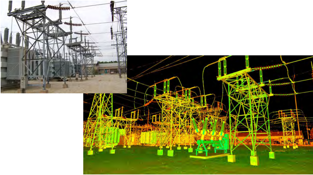
Figure 15-9: A photograph (upper left) and three-dimensional LiDAR data set, recording precise coordinates at a very high resolution. These coordinate data are useful for inspection, engineering, and maintenance, and were usually unavailable, or quite expensive, prior to LiDAR (courtesy Landpoint).
