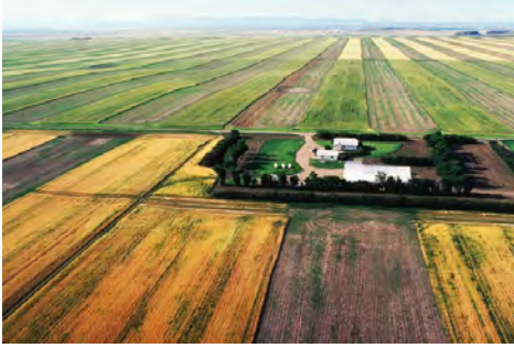
Figure 6-16: An example of tilt convergence. Crop bands of equal width appear narrower towards the horizon in this highly tilted image (courtesy USDA).
