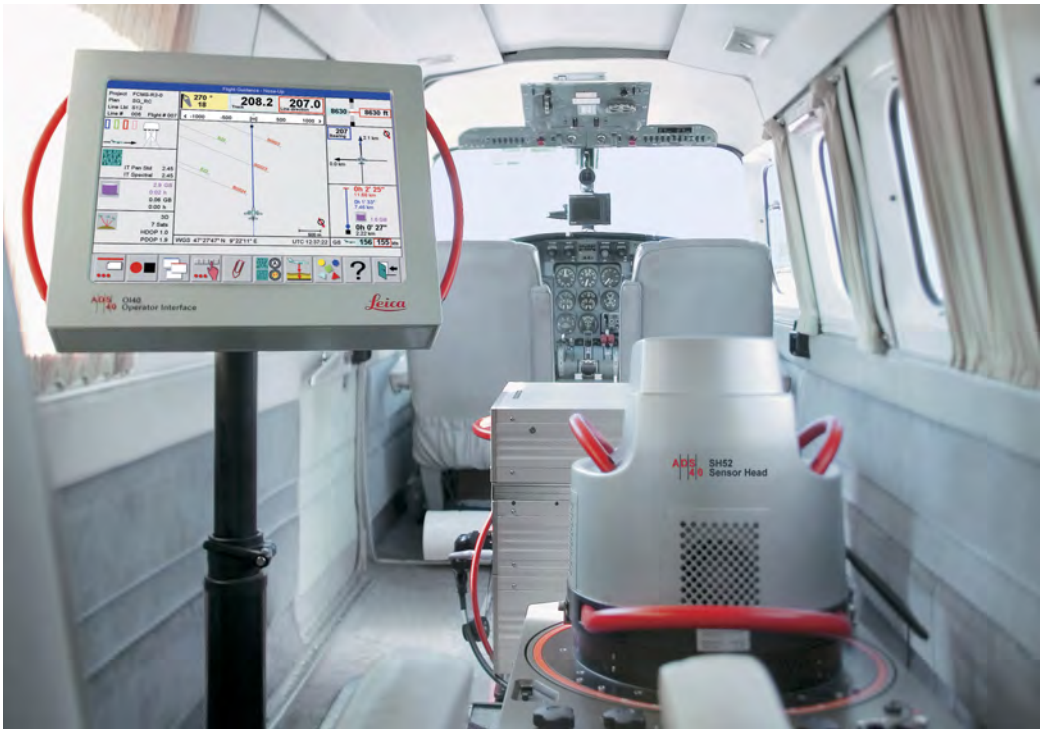
Figure 6-12: An example of the sophisticated system (upper left) for controlling digital image collection, here with a Leica Geosystems ADS40 digital aerial camera (lower right). These systems record and display flight paths and camera stations in real time, and may be used to plan, execute, and monitor image data collection (courtesy Leica Geosystems).
