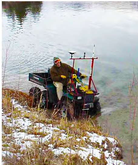
Figure 5-28: Line features may be field digitized via GPS, as in this example of a GIS/GPS system mounted in a tractor. Data display and digitizing software are used to record coordinates collected by a GPS receiver (above). An antenna placed on a pole or rack (right) reduces obstruction (courtesy Jake Leguee, left, and G. Johnson, Ducks Unlimited, right).
