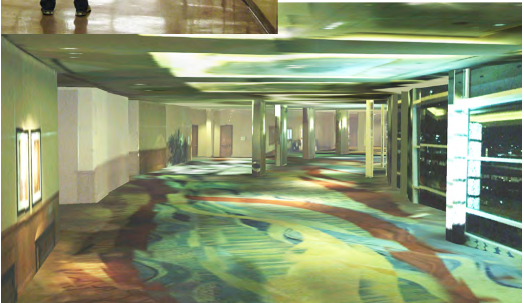
Figure 15-12: An example of indoor, three-dimensional data acquisition and organization. Image and LiDAR data collected with a backpack system (top) provide three-dimensional reconstructions of indoor environments (middle). These may be combined, maintaining accurate absolute position, to reconstruct connected building interiors (bottom). While currently an active research area, progress is apparent in applications, and will accelerate as data collection, storage, processing, and analysis hurdles are overcome, and as standards are established for data storage and access (courtesy Avidah Zakhori, U.C. Berkeley Video and Image Processing Lab).
