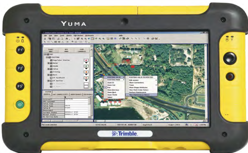
Figure 5-30: Features may be entered and edited in the field using a GPS receiver and appropriate software (courtesy Trimble, Ltd.).
