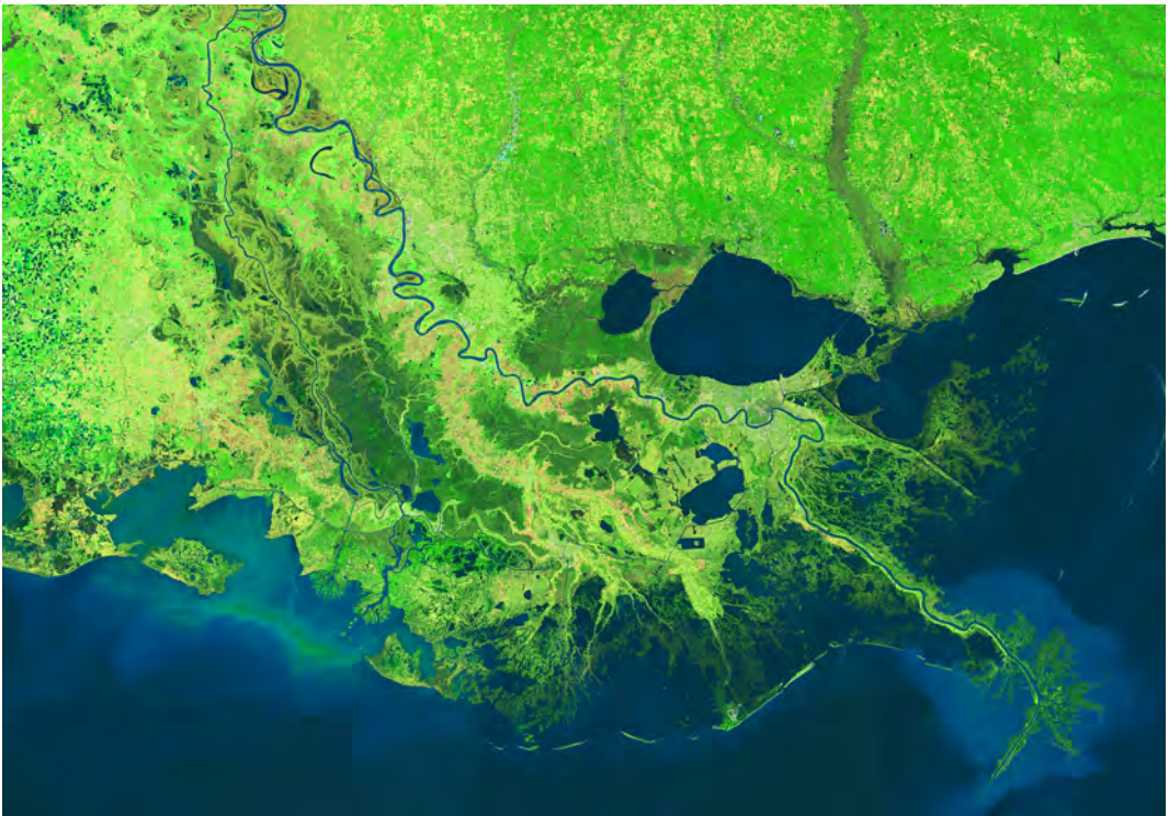
Figure 6-32: An example of a Landsat-5 image, showing the Mississippi River Delta. Mid-resolution satellites are particularly appropriate for regional or other large-area analysis (courtesy NASA).
