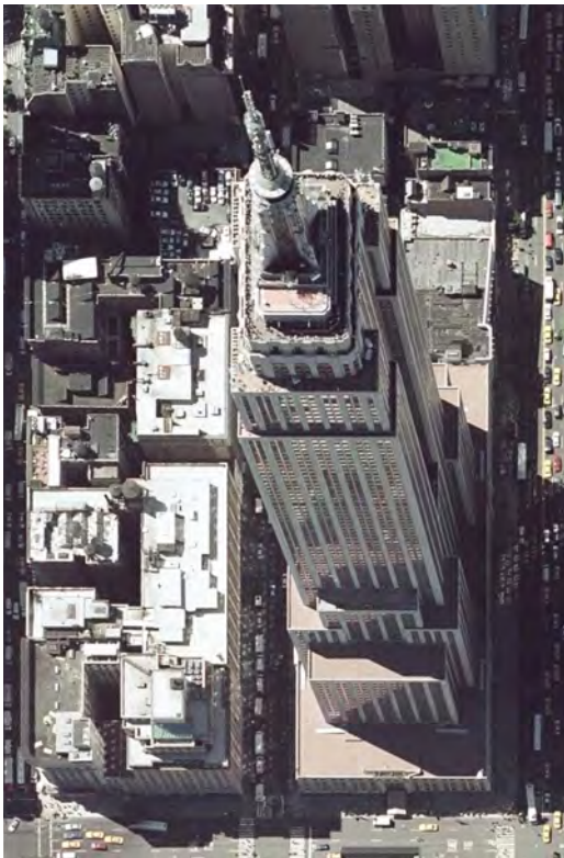
Figure 6-13: Tilt distortion is common on aerial and some satellite images, the result of perspective distortion when imaging the top and bottom of buildings, or any objects at different elevations.
