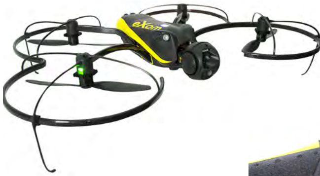
Figure 15-10: UAVs fitted with cameras and advanced GNSS may collect millimeter-accuracy spatial data from aerial imagery (courtesy senseFly).
