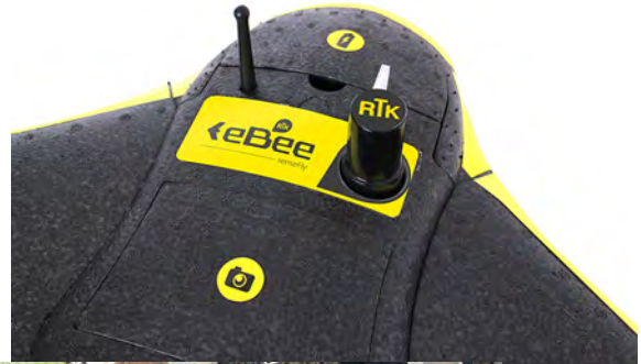
Figure 15-10: UAVs fitted with cameras and advanced GNSS may collect millimeter-accuracy spatial data from aerial imagery (courtesy senseFly).
