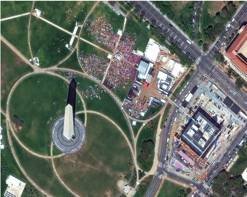
Figure 15-8: An image from the Worldview-3 satellite, taken over Washington, D.C. This satellite produces up to 25 cm resolution images, and is soon to be joined by others of the same high resolution. We may soon have daily, global, high-resolution images (courtesy DigitalGlobe).
