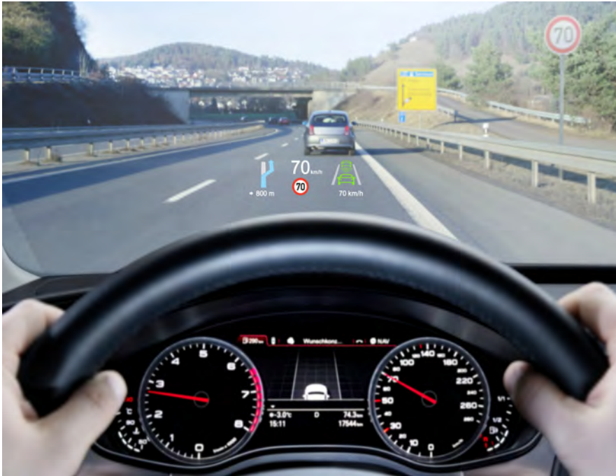
Figure 15-6: Heads-up displays may appear in autos, improving driver safety and trip efficiency under inclement weather (courtesy Continental).
