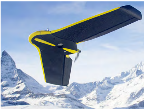
Figure 6-41: The senseFly ebee, and example of small UAV/drones optimized for spatial data collection (courtesy senseFly Ltd.).
