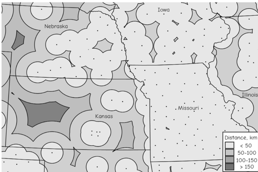
Figure 5-17: The location of RTK available stations (dots) in the central U.S. in April, 2015. Station locations and distances from the nearest beacon are shown.
