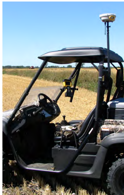
Figure 5-4: A hand-held GNSS receiver (left) and a GNSS receiver in use (right), (courtesy Topcon, and G. Johnson).
