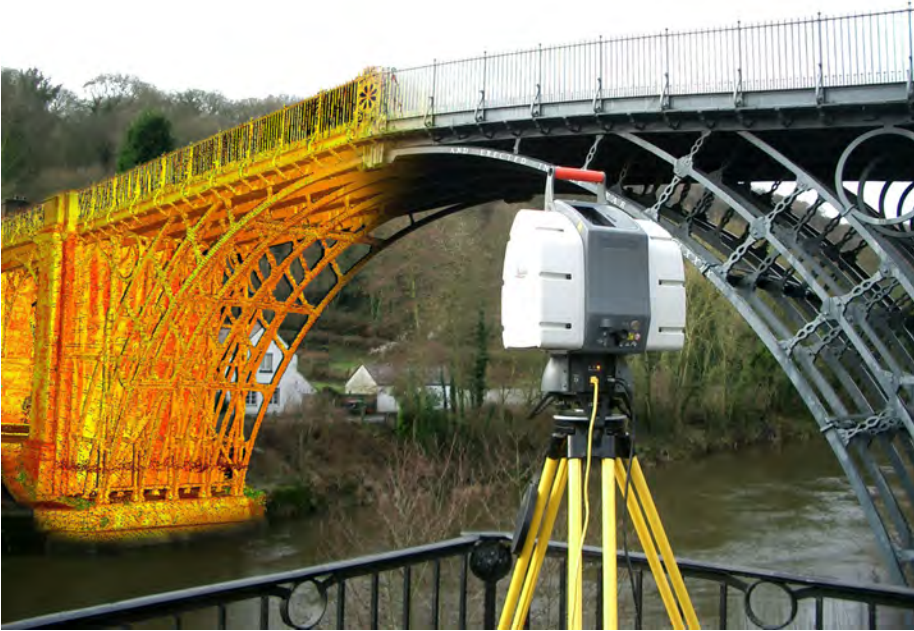
Figure 5-26: Three-dimensional scanning lasers use coordinate geometry to record comprehensive x, y, and z coordinate data for GIS. Here, a scanning laser is shown (foreground) with a portion of a the 3-D laser measurements (left) superimposed on the bridge (right). Courtesy Leica Geosystems.
