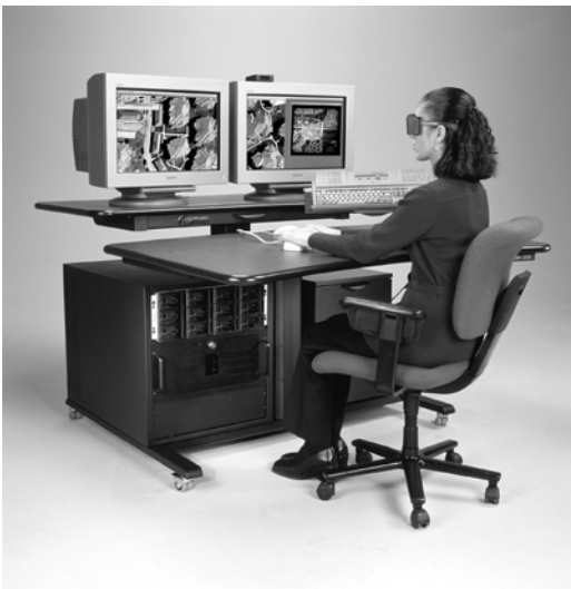
Figure 6-24: A softcopy photogrammetric workstation, used in the production of orthophotographs (courtesy Z/I Imaging Systems).
