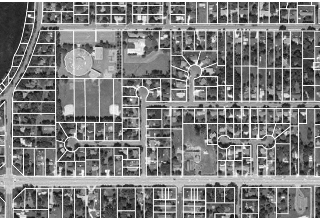
Figure 5-19: Surveying establishes the coordinates for most property lines. Field measurements of distance and direction are used to establish the set of vertices that define property boundary lines. This is the only way to collect these data, as the features are not visible on any other source.
