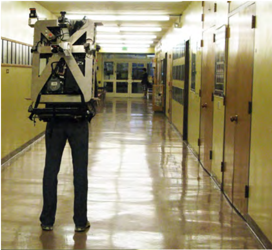
Figure 15-12: An example of indoor, three-dimensional data acquisition and organization. Image and LiDAR data collected with a backpack system (top) provide three-dimensional reconstructions of indoor environments (middle). These may be combined, maintaining accurate absolute position, to reconstruct connected building interiors (bottom). While currently an active research area, progress is apparent in applications, and will accelerate as data collection, storage, processing, and analysis hurdles are overcome, and as standards are established for data storage and access (courtesy Avidah Zakhori, U.C. Berkeley Video and Image Processing Lab).
