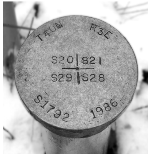
Figure 3-52: A PLSS corner that has been surveyed and marked with a monument. This monument shows the physical location of a section corner. These points are often used as control points for further spatial data development.
