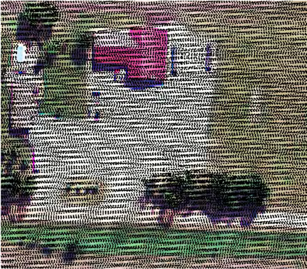
Figure 6-39: LiDAR sampling pattern, each dot represents a lidar return. Scan lines overlap, resulting in an uneven distribution of returns at very fine scales. Results are usually summarized for raster cells or areas that span gaps.
