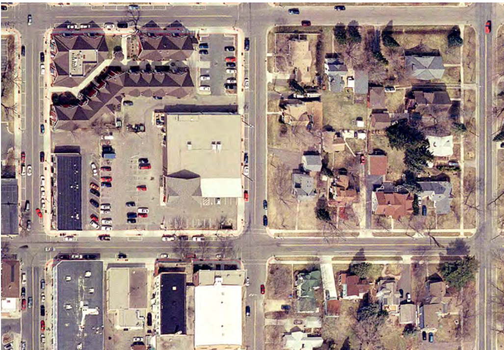
Figure 6-8: Digital images may provide image quality equal to or better than film images. This figure shows images collected at 15 cm resolution. Extreme detail is visible, including roof vents, curb locations, and street poles (courtesy USGS).
