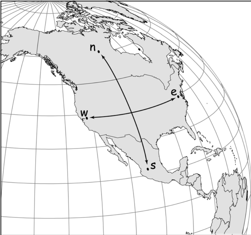
Figure 3-6: Two arcs illustrate the surface measurements and calculations used to estimate the semi-major and semi-minor axes, here for North America. The arc lengths may be measured by surface surveys, and the angles from astronomical observations, as illustrated in Figure 3-2 and Figure 3-3.
