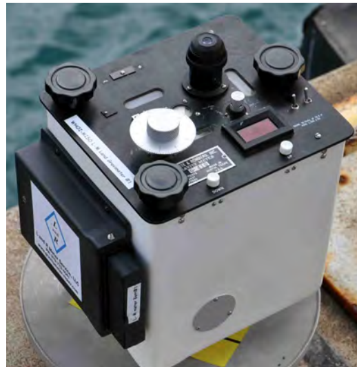
Figure 3-11: A portable field gravimeter, an instrument used for measuring gravitational force at a field location. These measurements are combined with surveying measurements to estimate geoidal surfaces (courtesy NOAA).
